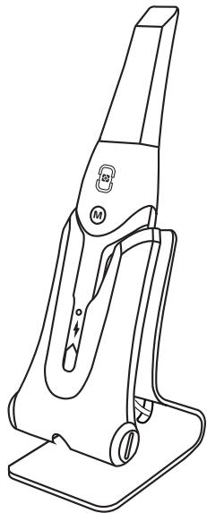
**NOTE:** The scanner will automatically shut down if it is idle for more than 3 minutes. If you need to use it again, press any button on the scanner, or take it out of the Charging Holder.
